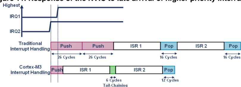
Similarly, the NVIC abandons a stack Pop if an exception arrives and services the new interrupt immediately. By pre-empting and switching to the second interrupt without completing the state restore and save, the NVIC achieves lower latency in a deterministic manner.
